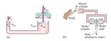
(a) Hydraulic lift: A device that <u>lifts a car</u> using a small force applied over <u>a larger area</u>.
